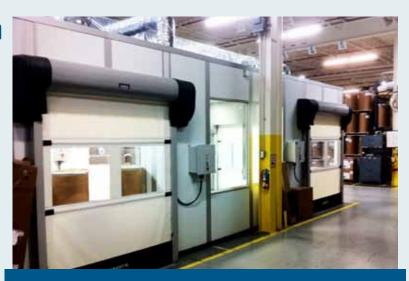
Our distributor provided Mallinckrodt Pharmaceuticals with a new product sampling booth at their manufacturing facility located in Greeneville, IL. The enclosure would provide their client with a temperature and humidity controlled area in which to inspect and re-package incoming products to ensure product quality.
