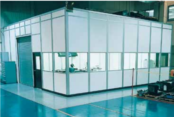
Environmentally-controlled CMM room with roll-up access door.
