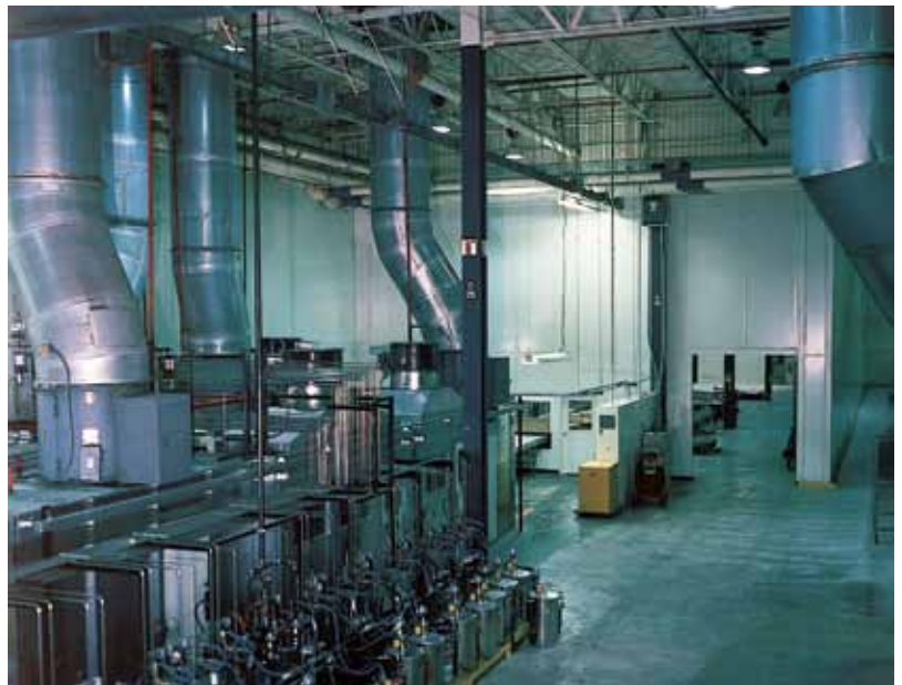
Finishing system enclosure enables control of temperature, humidity and particulates.
