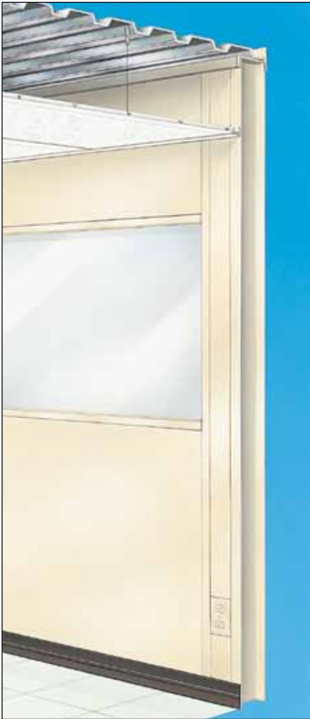
Ceiling suspended from roof deck.
